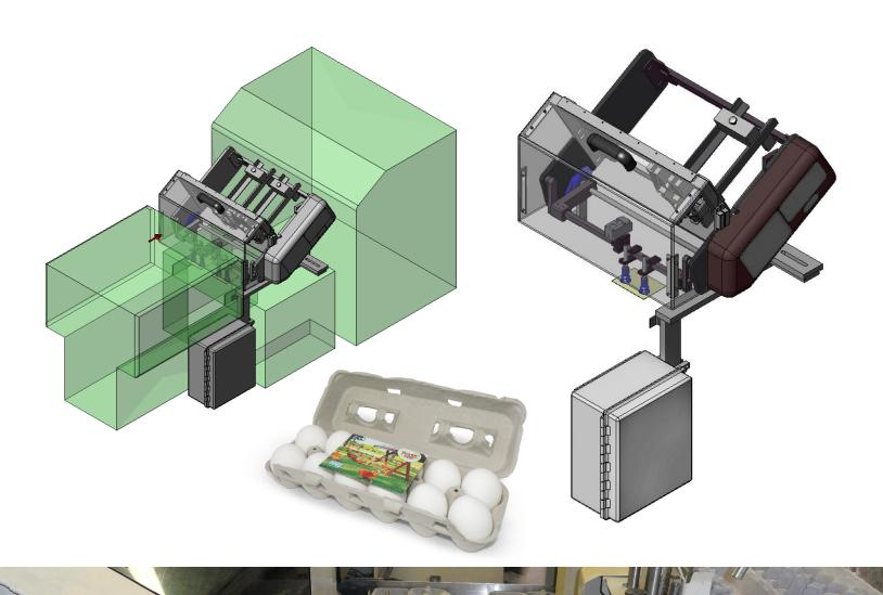
Proven System for Placing Labels Inside of Egg Cartons While Cartons are in Motion in an Egg Grading Machine.
